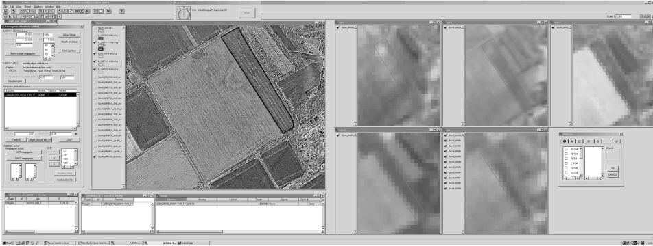
Figure 4: A screenshot of the Computer-Aided Photo-Interpretation software. (Large window on the left: VHR image, small windows: HR image time series)
