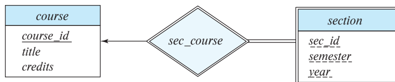
Figure 6.14 E-R diagram with a weak entity set.
