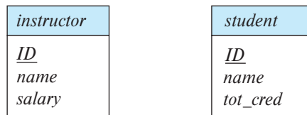
Figure 6.1 E-R diagram showing entity sets instructor and student .
