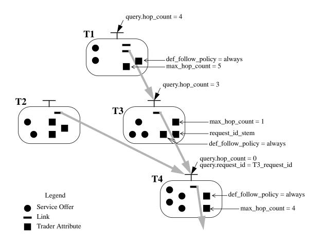
*Figure 1-4* Flow of a query through a trader graph
