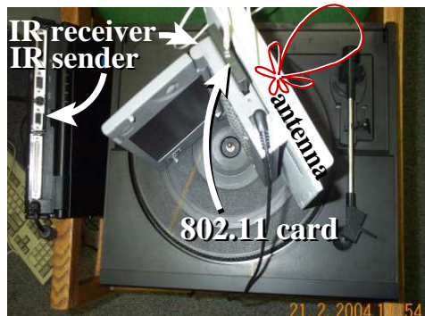
Figure 2: Experimental base station with revolving antenna
