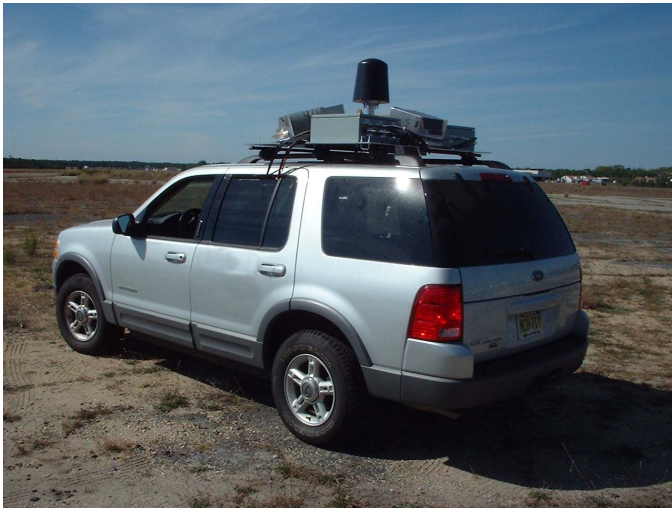
Fig. 8. Demo 2 Vehicle. Mounted on the roof are three high-band antennas and amplifiers in three 120-degree spaced boxes. There is also a low-band switching matrix and the lowband antenna. For this second demo, the lowband was changed to a “gumdrop” antenna that contained 5 antennas pointing front, back, left, right and up.
